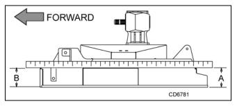
Figure 4. Cutting Height Adjustment
